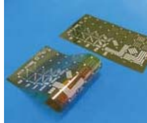
Production of FPCs through PE using silver paste
